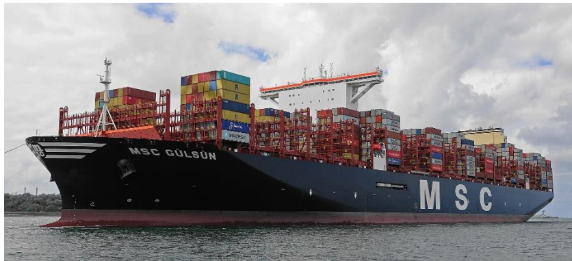
Pictures of MSC Gülsün ULVC container vessel Length over all (Loa): 399.9 m, Beam: 61.8 m, Draught: 16.5 m, Gross Tonnage (GT): 232618, Deadweight DWT: 228149
