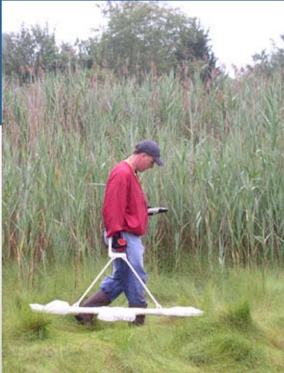
The Profiler EMP – 400 is a frequency domain, electromagnetic profiling system. By acquiring multiple frequencies, the user can select the frequencies that provide the best results for a specific application.
