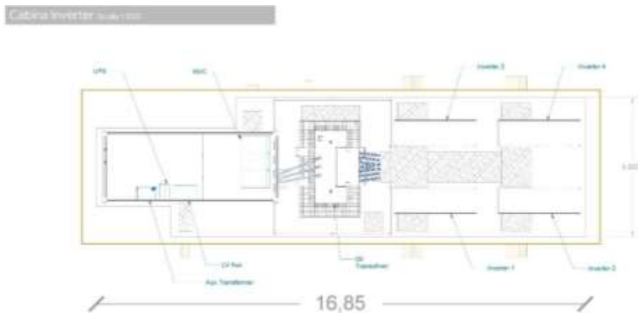
Figura 60: Power station 4 inverters
