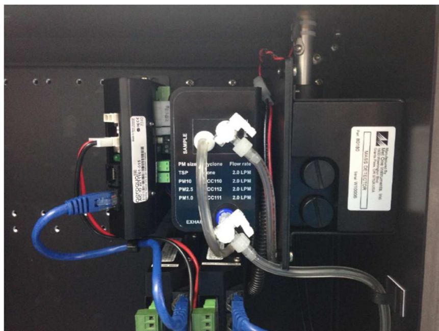
Figure 12-4 The Particle Monitor uses three modules: a) the optical engine on the far right, b) the pump module in the middle, c) the I/O module on the left (configuration is subject to change)
