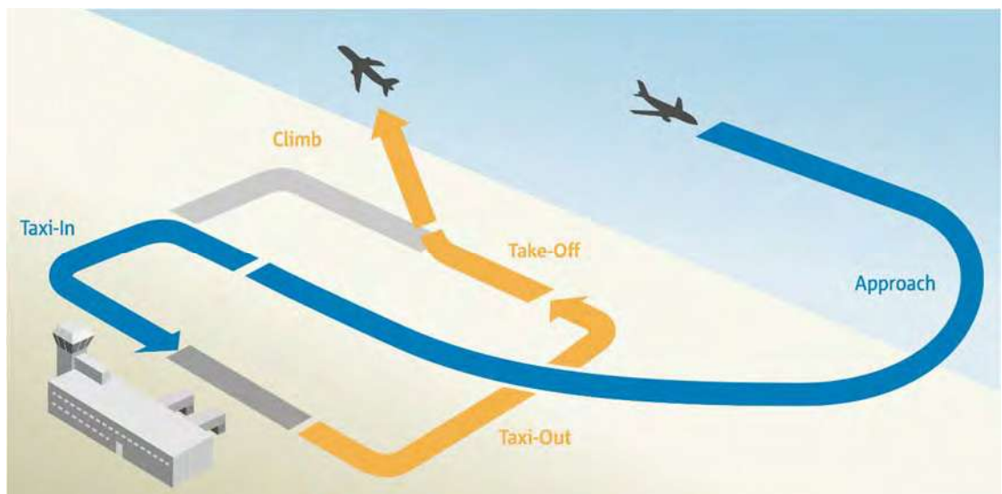
Figura 4-2 - LTO cycle from European Environment Agency, European Union Aviation Safety Agency, "European aviation environmental report 2016", Publications Office of the European Union, 2016, https://data.europa.eu/doi/10.2822/385503 .
