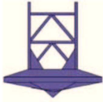
Figura 4.3: Spudcan - Profilo Tipico (Bennet& Associates e Offshore Technology, 2005)
