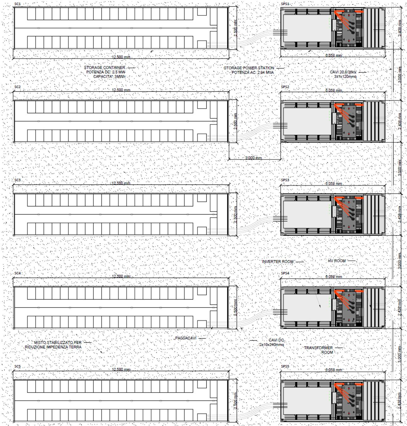
Figura 3: Dettaglio storage container e storage power station
