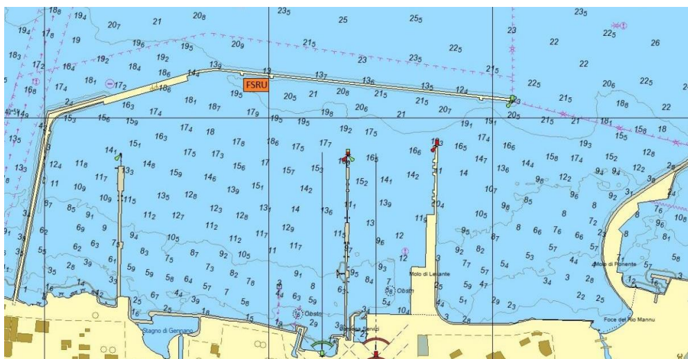
Figura 3-3 – Dettaglio della batimetria (Rif. Database CM-93/3, DHI, "MIKE C-MAP, Extraction of the World Wide Bathymetry Data and Tidal Information, Scientific Documentation" MIKE by DHI, Horsholm 2021).
