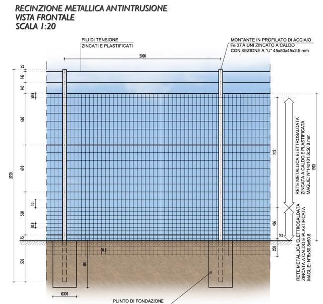
RECINZIONE METALLICA TIPO R.1.B. COSTITUITA DA RETE ELETTROSDATA A MAGLIA DIFFERENZIATA SOSTENUTA DA PALI AD U IN ACCIAIO ZINCATO, SOSTEGNI E FILI DI TENSIONE.
