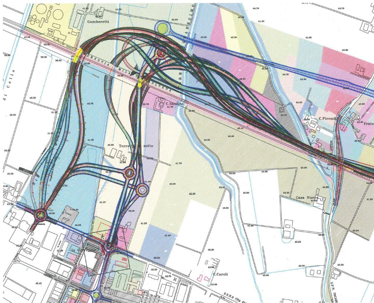
FIGURA 4.1-1 – SOVRAPPOSIZIONE ALLO STRUMENTO URBANISTICO LOCALE DI TUTTE LE ALTERNATIVE STUDIATE PER IL NODO DI CORTE TEGGE
