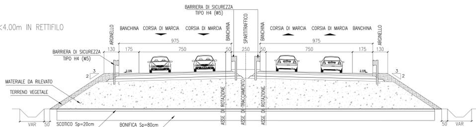
B 2+2 IN RILEVATO H>4.00m IN RETTIFILLO
