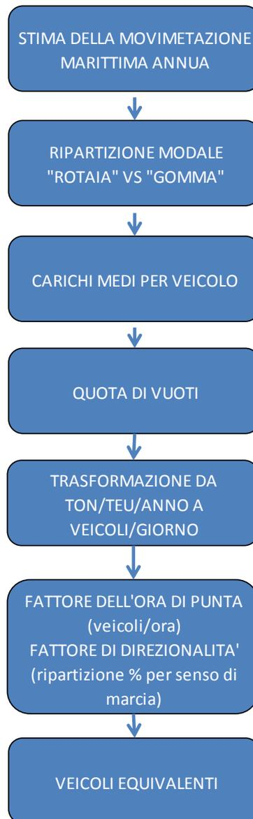
FIGURA 9-4 – STEP METODOLOGICI PER IL CALCOLO DEI FLUSSI STRADALI
