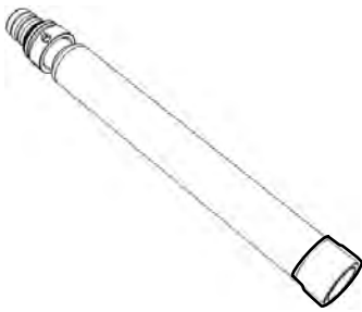
Figure 61 Turbidity sensor storage
