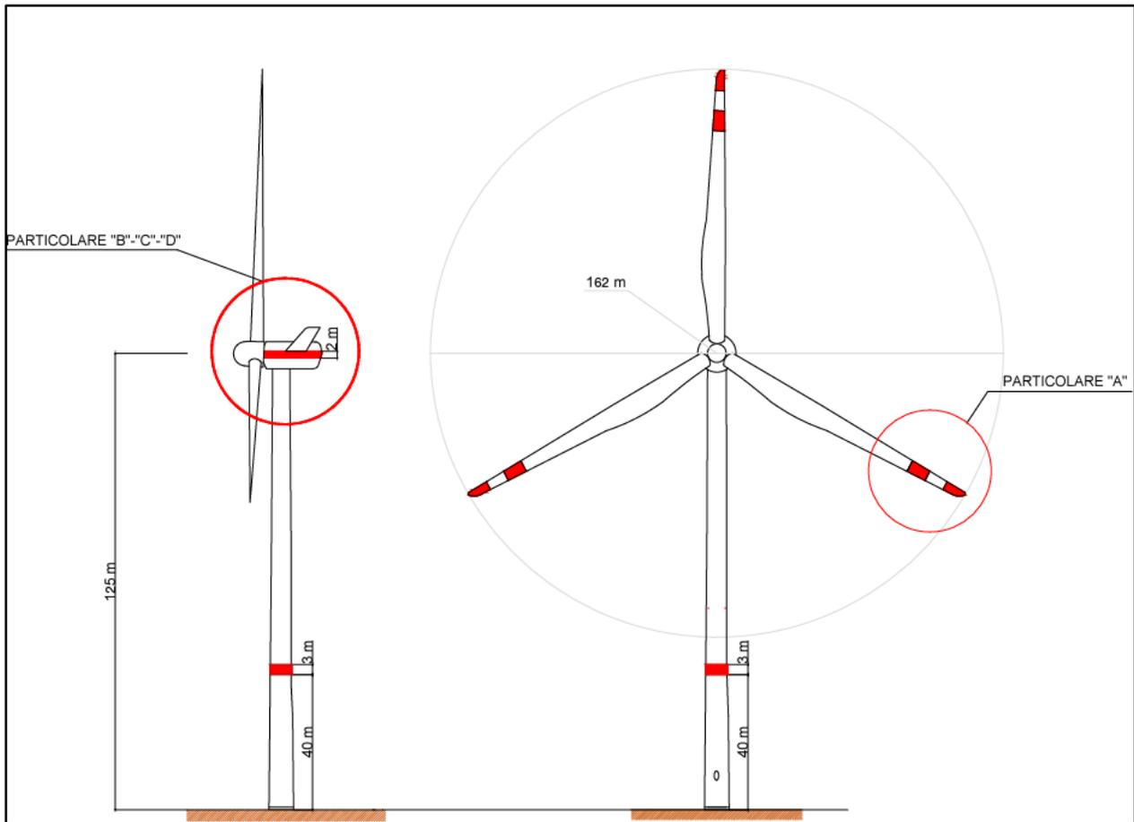
Figura 4.1: Profilo aerogeneratore V162 – 6,0 MWp – HH = 125 m – D = 162 m
