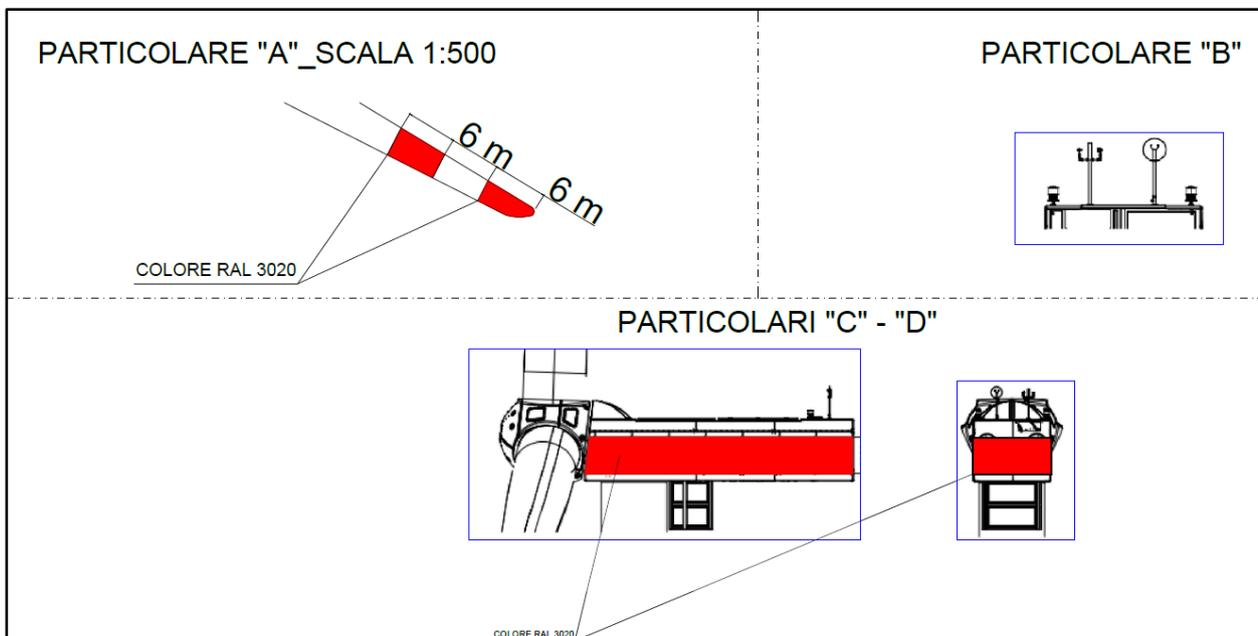
Figura 4.2: Particolari aerogeneratore V162– 6,0 MW – HH = 125 m – D = 162 m
