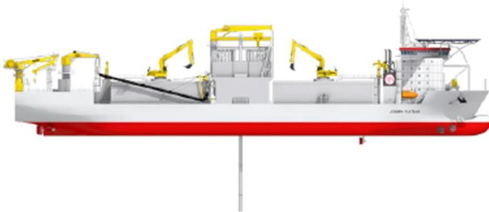
**Figura 7.5: Tipico Fall Pipe Vessel**
