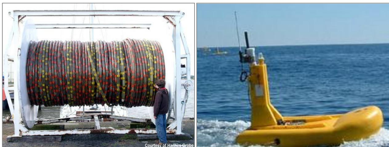
Figura 2.7 – *Streamer* o cavo sismico per l'acquisizione a sinistra (fonte: [www.offshore-technology.com/features/feature43561/feature43561-3.html](http://www.offshore-technology.com/features/feature43561/feature43561-3.html)) e *Boa di coda* a destra (fonte: [www.seamap.com](http://www.seamap.com)).
