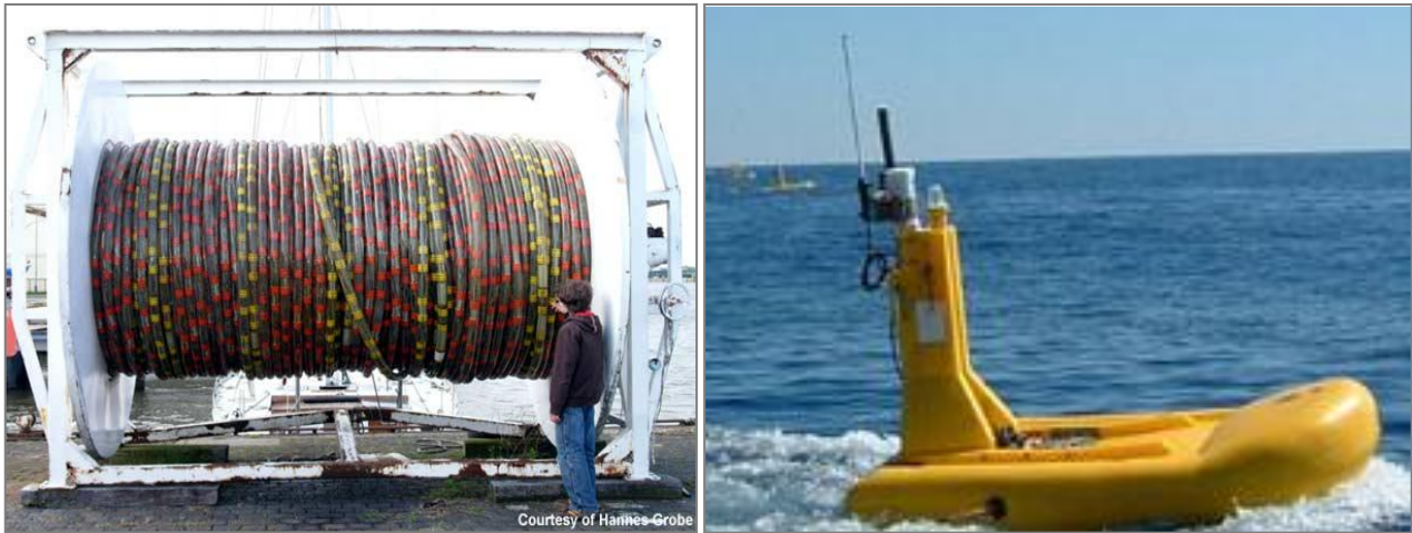
Figura 2.7 – Streamer o cavo sismico per l’acquisizione a sinistra (fonte: www.offshore-technology.com/features/feature43561/feature43561-3.html ) e Boa di coda a destra (fonte: http://www.seamap.com/products/seismic/buoylink/ )
