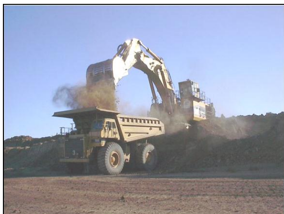
Figura 55 Truck Loading: Overburden SCC 05-010-37
