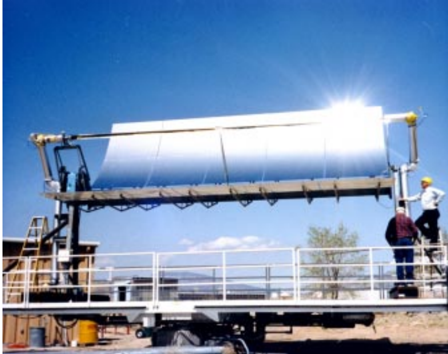
Figure 3. An LS-2 collector was tested on SNL's rotating platform. The platform allows the collector to be pointed directly at the sun at all times of the day.
