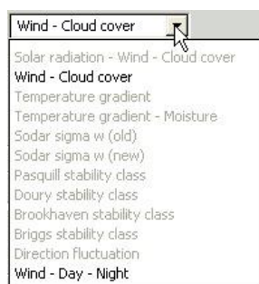
Figure 40: Methods for calculating stability class
