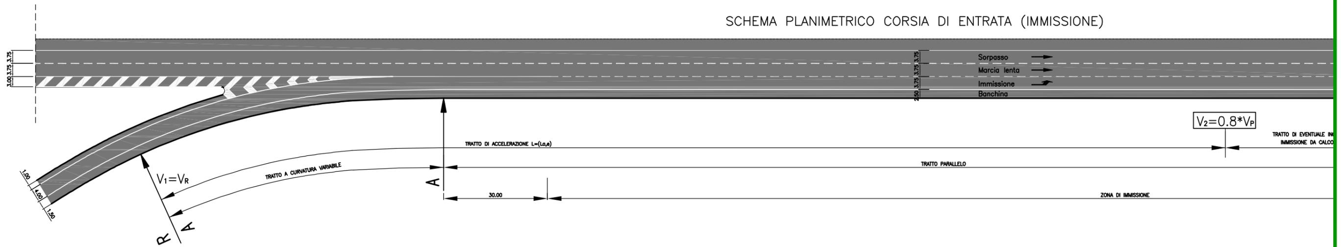
$$L_{d,u} = \frac{V_1^2 - V_2^2}{2a} \quad L_{a,e} = \frac{V_2^2 - V_1^2}{2a}$$
