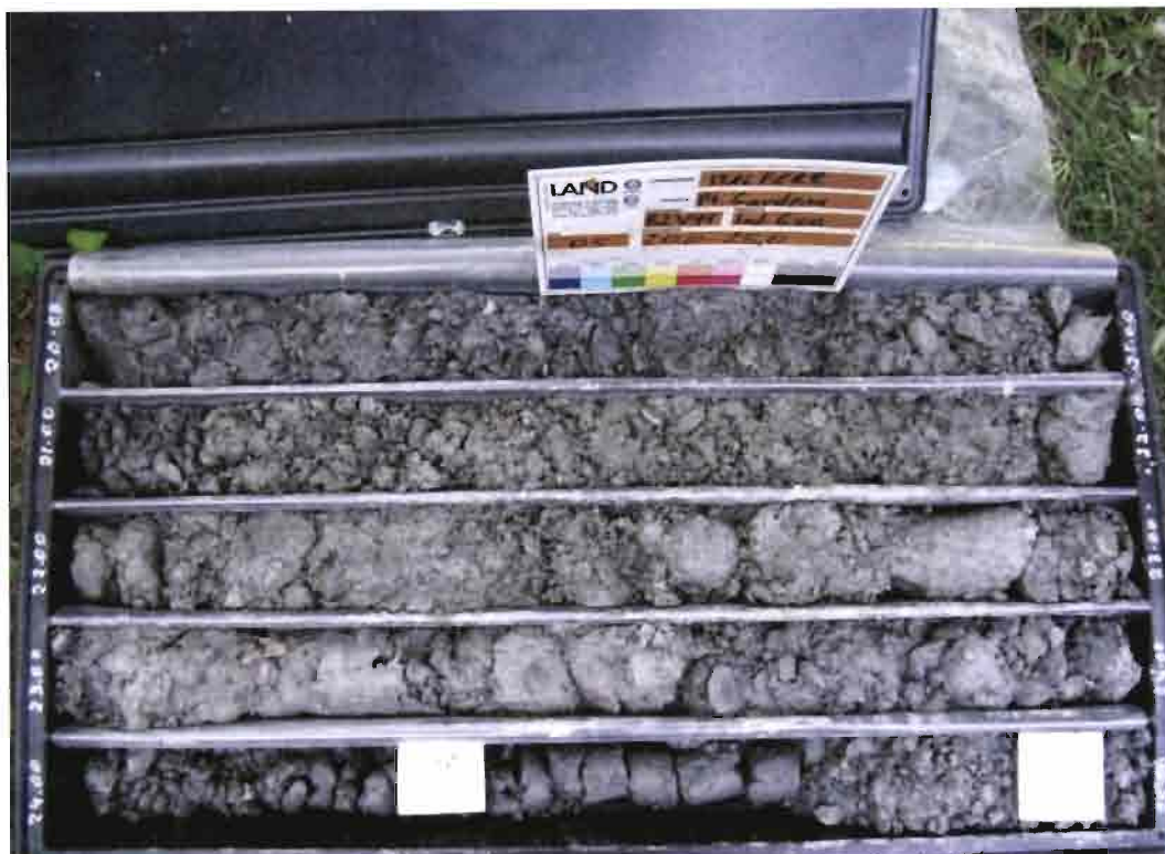
Ponte Gardena (BZ) - B2V11 - Box 5 - m 20.00 ÷ m 25.00
