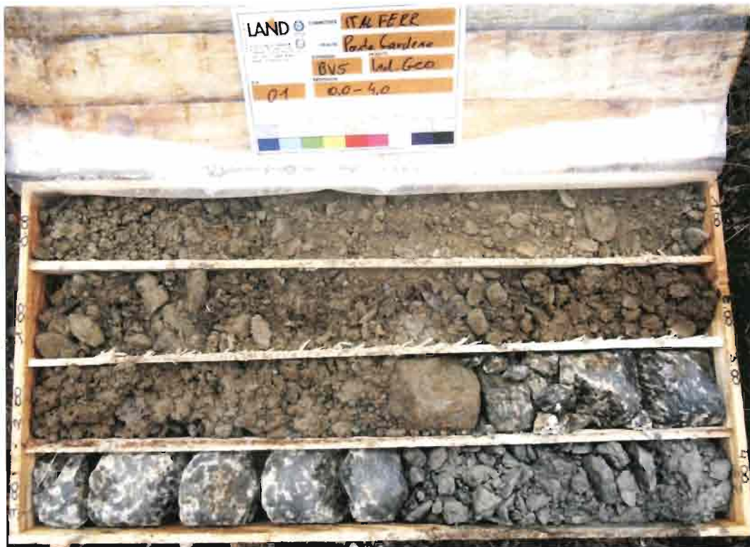
Ponte Gardena (BZ) - BV5 - Box 1 - m 0.00 ÷ m 4.00
