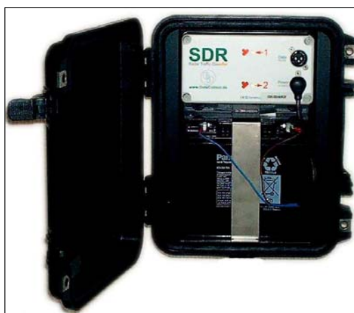
Contatraffico Radar SDR Easydata
