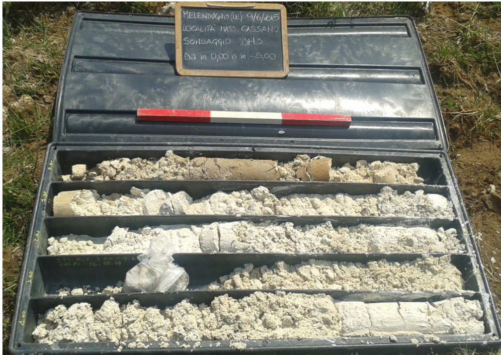
Figure 1: Borehole BH3 - (0.00 ÷ 5.00 m)
