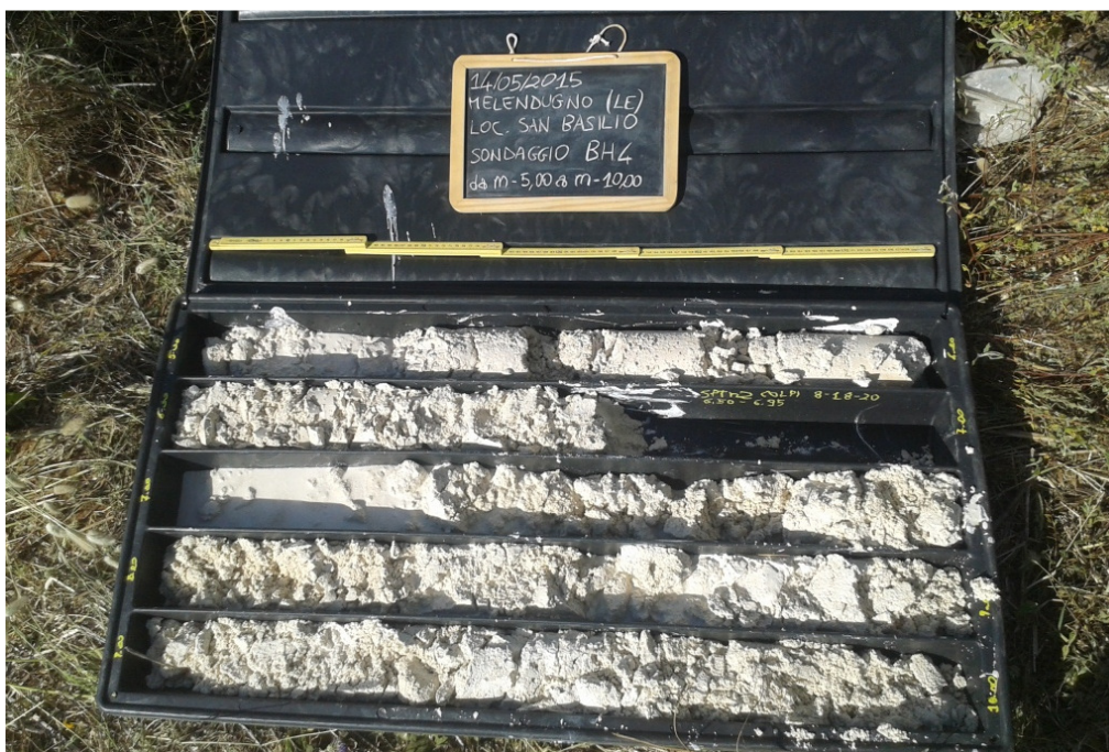
Figure 4: Borehole BH4 - (5.00 ÷ 10.00 m)
