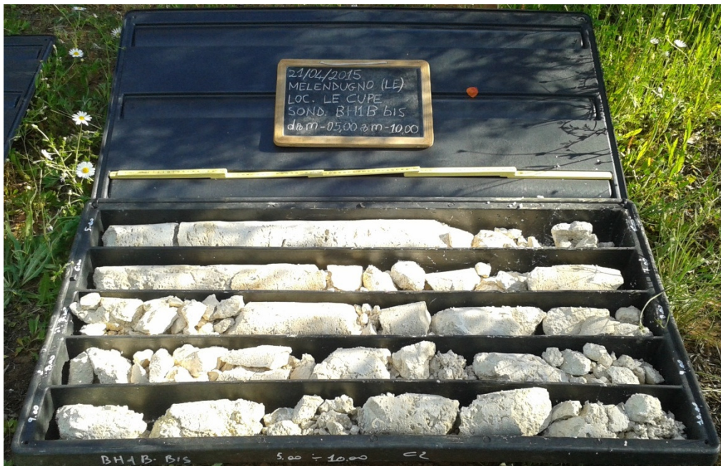
Figure 38: Borehole BH1Bbis - (5,00 ÷ 10,00 m)
