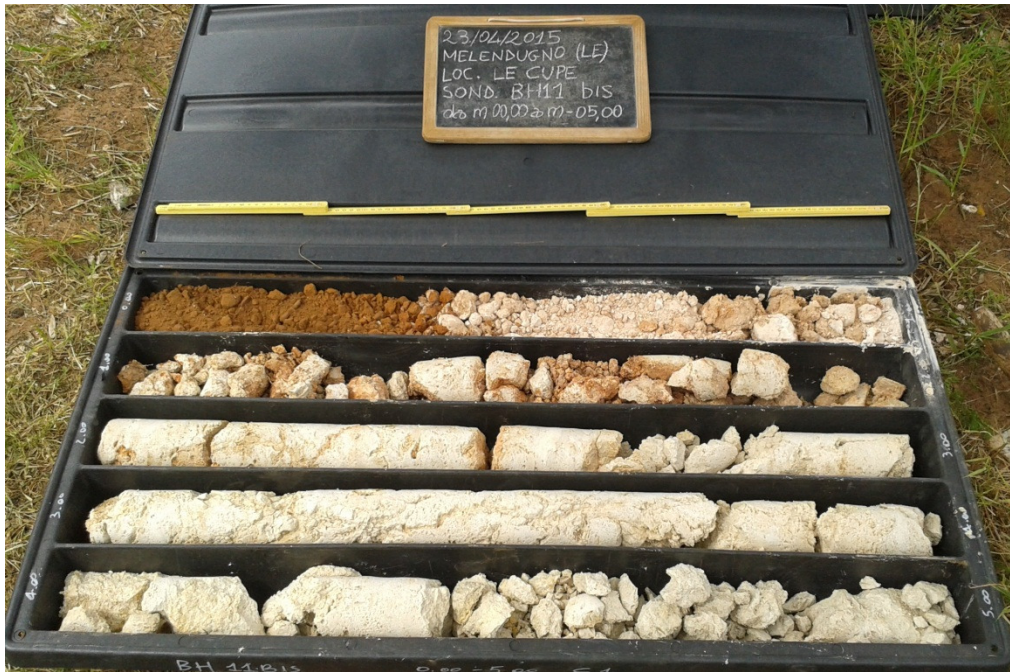
Figure 31: Borehole BH11bis - (0,00 ÷ 5,00 m)
