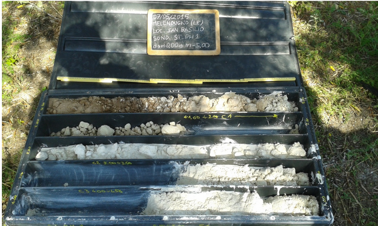
Figure 5: Borehole ST_BH1 - (0,00 ÷ 5,00 m)
