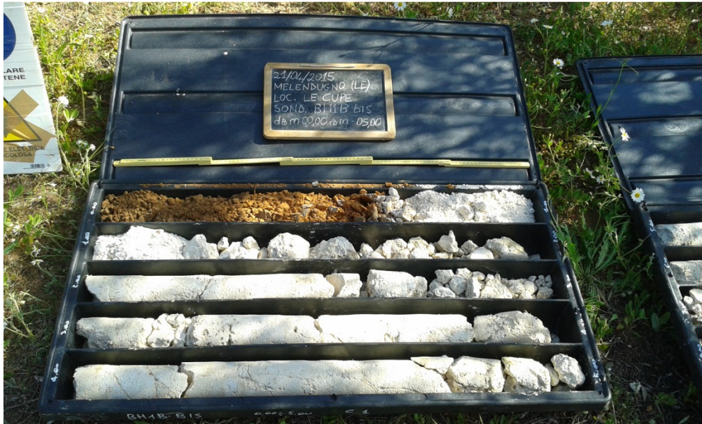
Figure 37: Borehole BH1Bbis - (0,00 ÷ 5,00 m)
