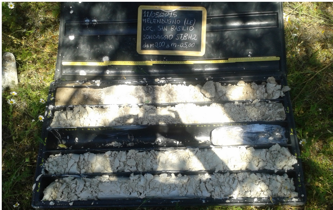
Figure 1: Borehole ST_BH2 - (0,00 ÷ 5,00 m)
