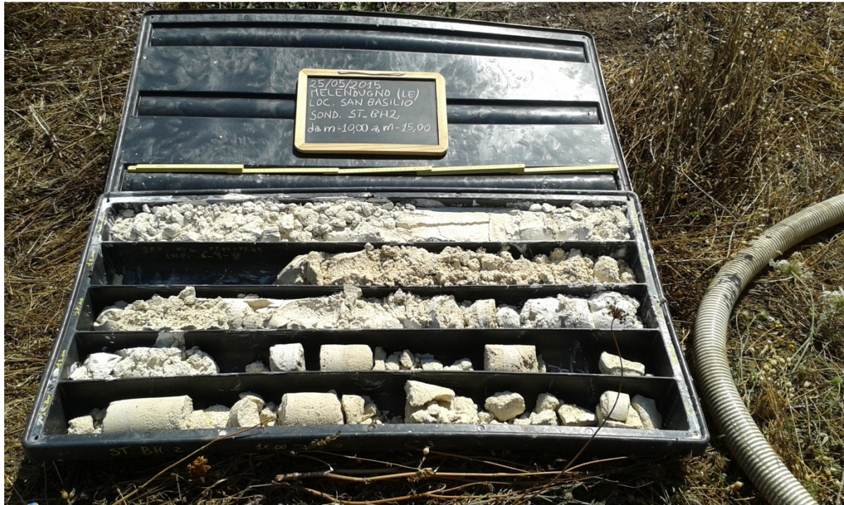
Figure 3: Borehole ST_BH2 - (10,00 ÷ 15,00 m)
