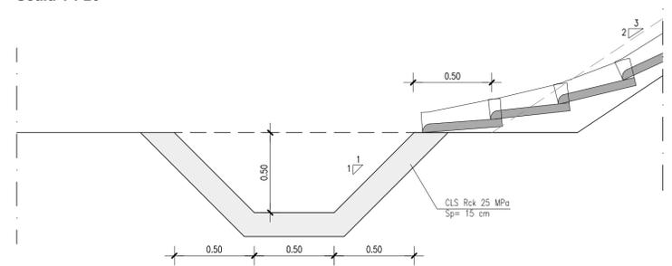
**PARTICOLARE SEMITUBO IN CLS PER RACCOLTA ACQUE A TERGO MURO**
