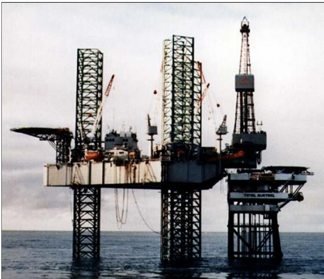
Figura 3-8: Jack-up Drilling Unit
