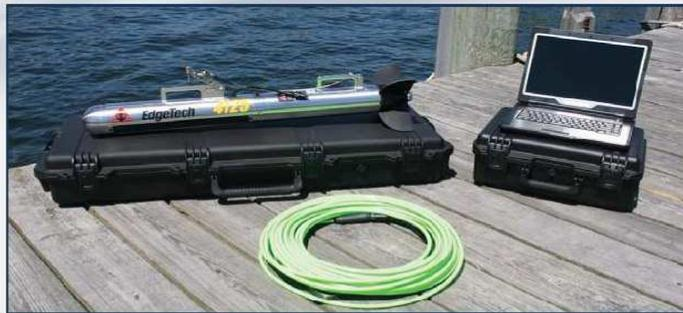
EdgeTech's 4125 Side Scan Sonar System was designed with both the Search & Recovery (SAR) and shallow water survey communities in mind. The 4125 utilizes EdgeTech's Full Spectrum® CHIRP technology, which provides higher resolution imagery at ranges up to 50% greater than non-CHIRP systems operating at the same frequency. This translates into more accurate results and faster surveys, thus cutting down on costs.
