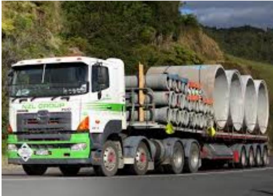
Fig. 8.4 – Transport and stacking of concrete pipes
