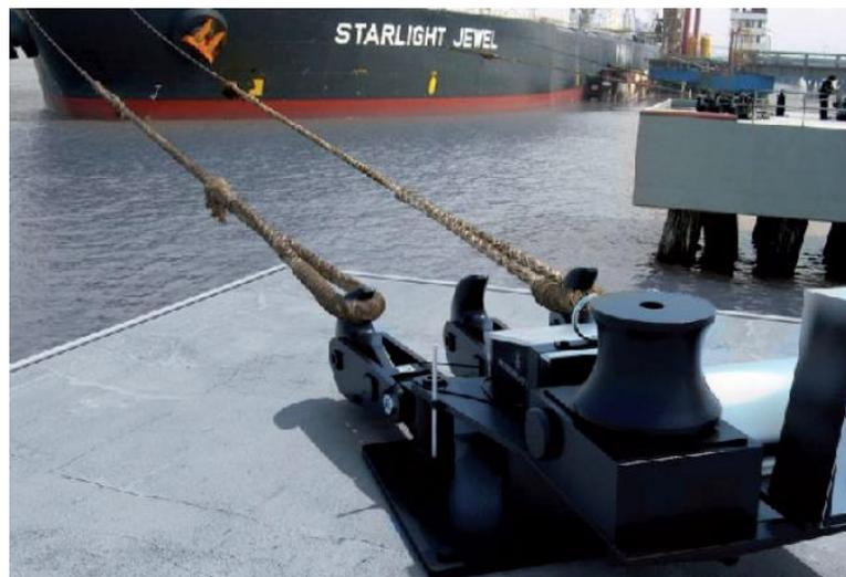
**Figura 4.3: Quick Release Hooks**
