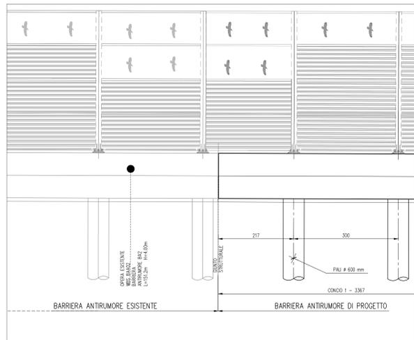
PROSPETTO BARRIERA DI PROGETTO IN CORRISPONDENZA DELL'USCITA DI SICUREZZA
