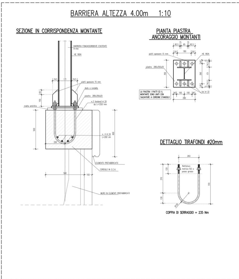
TIPOLOGICO PER BARRIERE SU MURO DI PROGETTO BA6
