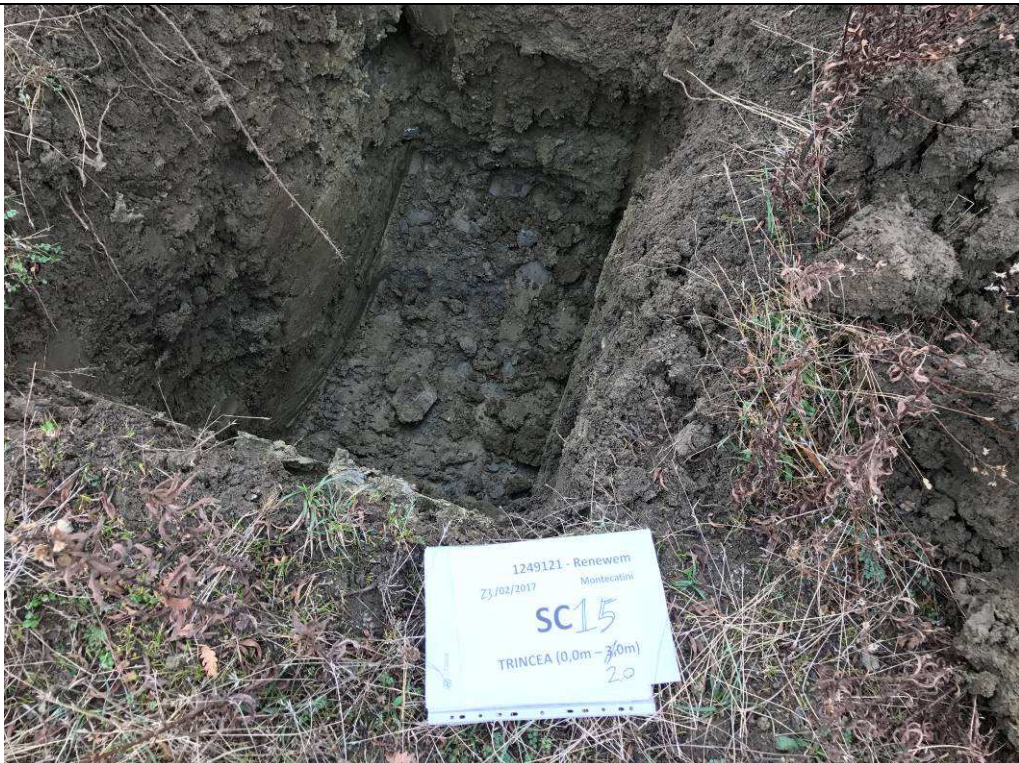
SC15 – Trincea (0,0-2,0) m p.c.
