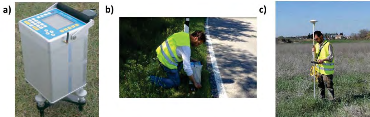
Fig. 11 - a) Scintrex CG-5. b) Example of gravity measurement. c) Example of GPS measurement.
