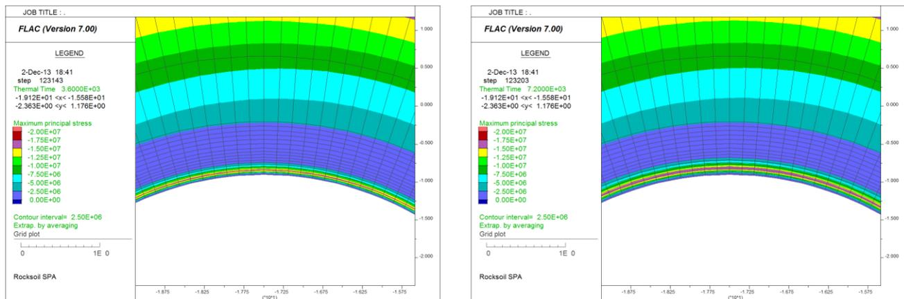
Figura 36 – Sigma 1 – Curva UNI11076 – t = 120 min
