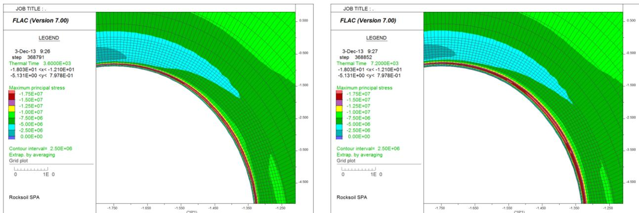
Figura 61 – Sigma 1 – Curva UNI11076 – t = 120 min
