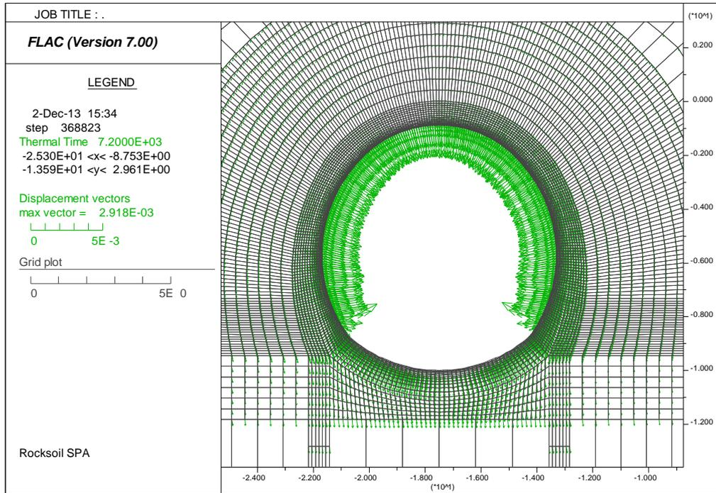
**Figura 54 – Deformata – Curva EUREKA – t = 120 min**
