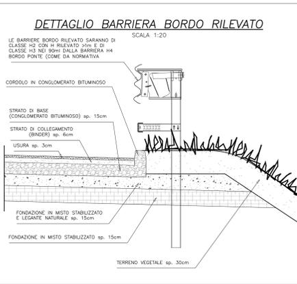
LE BARRIERE BORDO RILEVATO SARANNO DI CLASSE H2 CON H RILEVATO 20cm E DI CLASSE H3 NEI 90m DALLA BARRIERA H4 BORDO FONTE, COME DA NORMATIVA.
