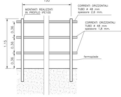
RINGHIERA IN ACCIAIO CLASSE Fe430 O SUPERIORE SECONDO NORMA UNI 7070, ZINCATA A CALDO SECONDO NORMATIVA UNI 5744
