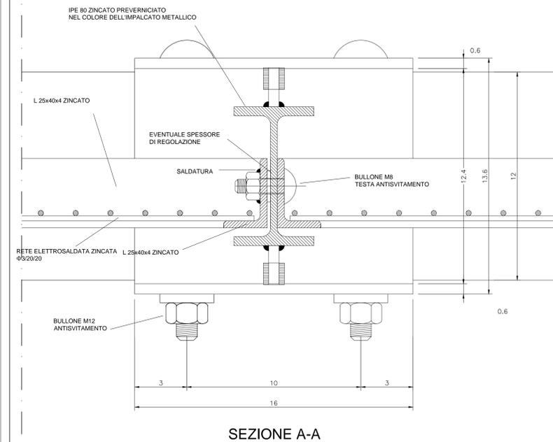
TELAJ REALIZZATI CON L 25x40x4 E RETE ELETTROSALDATA Ø3/20/20 mm
