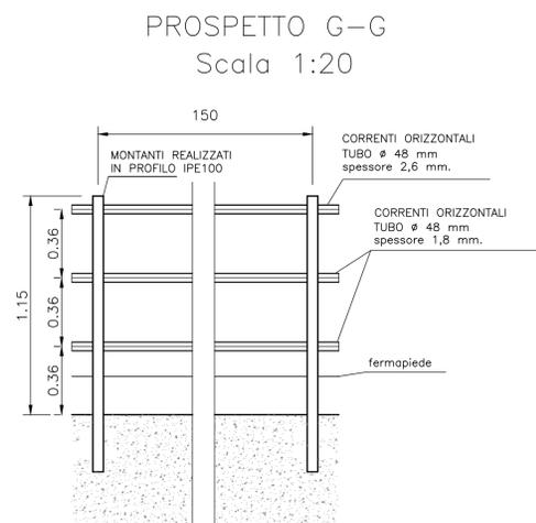
RINGHIERA IN ACCIAIO CLASSE Fe430 O SUPERIORE SECONDO NORMA UNI 7070, ZINCATA A CALDO SECONDO NORMATIVA UNI 5744
