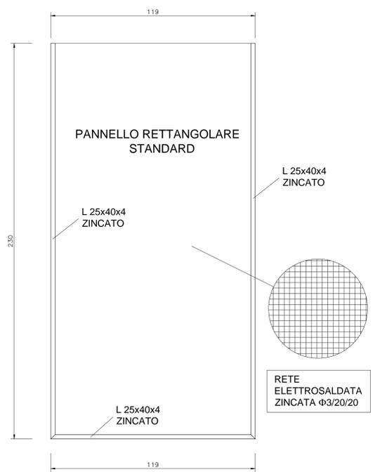
TELAI REALIZZATI CON L 25x40x4 E RETE ELETTROSALDATA Ø3/20/20 mm
