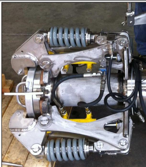
Figura 3 - Quick Connect / Disconnect Coupler
