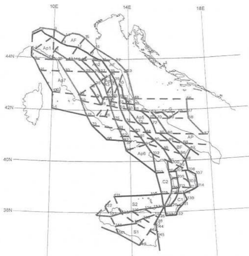
Figure 1. Morphostructural map of the study area. Violet lines are the lineaments of the first rank, blue lines are the lineaments of the second rank, green lines are the lineaments of the third rank, continuous lines are the longitudinal lineaments, discontinuous ones are the transverse lineaments. Nodes are numbered from 1 to 145. Ap, Apennines; AF, Adriatic foredeep; AP, Apulian platform; BF, Bradanic foredeep; C, Calabria; G, Gargano Promontory; S, Sicily.
