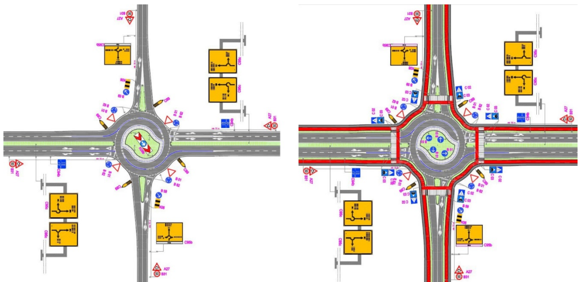
Figure 61: Overview of a turbo roundabout outside and within urban areas (Source: Guidelines for the design of roundabouts with the spiral flow the circular carriageway on State roads, 2014)
