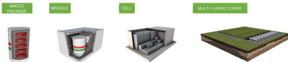
Figure 3.3-6: The engineering barriers of the National Repository
