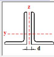
2 L 150 x 150 x 10    N<sub>by,Rd</sub> [kN]: 1 079    N<sub>bv,Rd</sub> [kN]: 695.9
