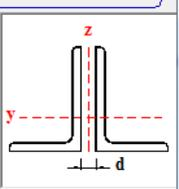
2 L 120 x 120 x 10    N<sub>by,Rd</sub> [kN]: 436.1    N<sub>bv,Rd</sub> [kN]: 206.0
