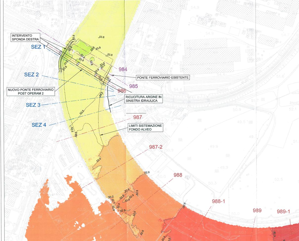
PLANIMETRIA LIVELLO IDRICO MASSIMO - SCENARIO INDISTURBATO - Scala 1:2'000
