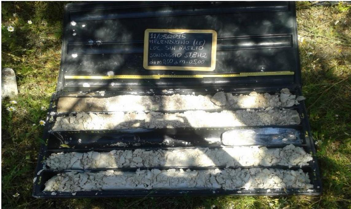
**Figura 7 – Sondaggio ST\_BH2: 0m – 5m (Rif.[9])**
