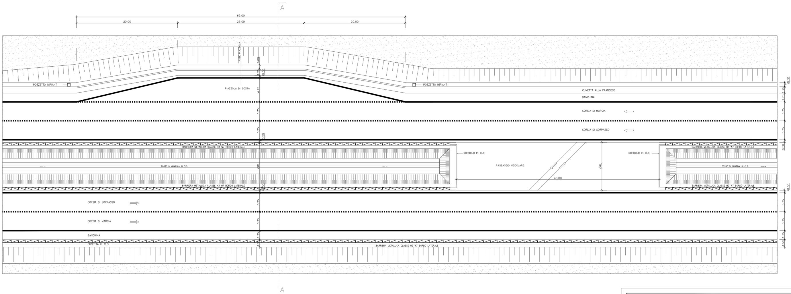
PARTICOLARE PIAZZOLA DI SOSTA E PASSAGGIO VEICOLARE TIPO - (PIANTA) SCALA 1:100
