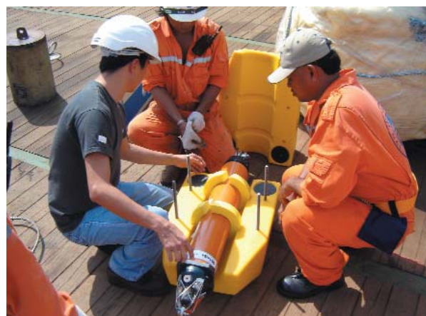
Transponder Options: Ranger 2 compatible transponders are available in a range of sizes, depth ratings, battery configurations and acoustic output power to suit deployment on subsea vehicles or on the seabed. (Above) Preparing a DPT transponder. (Below) New 6G® transponders.
