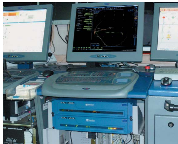
DP Reference: Ranger 2 installed in a DP desk. The system supports all industry stand DP telegrams, providing accurate and repeatable position referencing.
