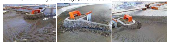
Undermining of the bridge parts to be build in the riverbed
